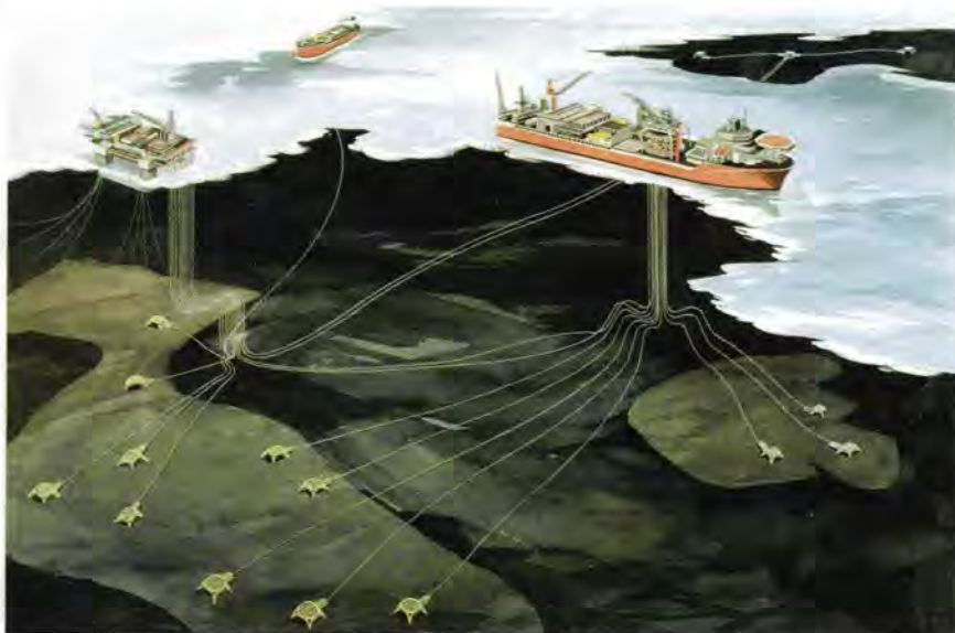
The Statoil-operated Åsgard field comprises the Åsgard A oil production vessel, the Åsgard C storage vessel and the Åsgard B gas platform.
