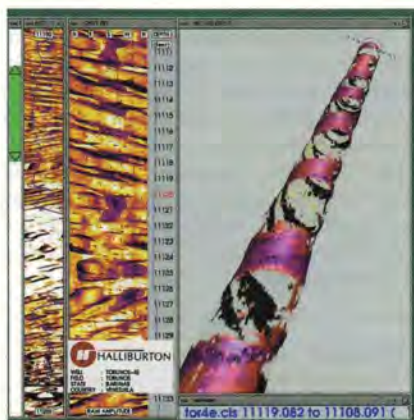
Figure 2: Spiral borehole as shown by the 2D (tracks 1 and 2) and 3D (track 3) images obtained from a wireline circumferential acoustic scanning tool (CAST™) in a well in Latin America. Note the spiral changed direction at a depth of 11,115 ft (3,388 metres) and had a pitch of 2 ft (0.61 metres).
