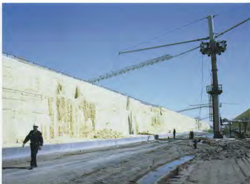
Over the years, Tengiz has accumulated 4.5mn tonnes of sulfur, storing it outdoors in huge slabs some 25 ft high and bigger than a football pitch
