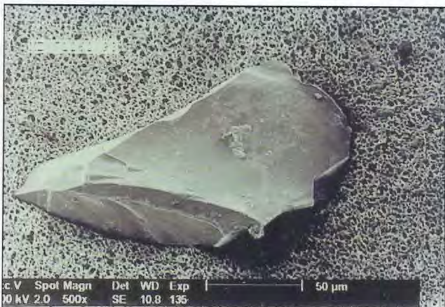
Figure 2: Electron micrograph of a metal fine – a tiny sharp piece of metal, like a tiny dagger that can scratch a worker's skin, the machine tool or component
