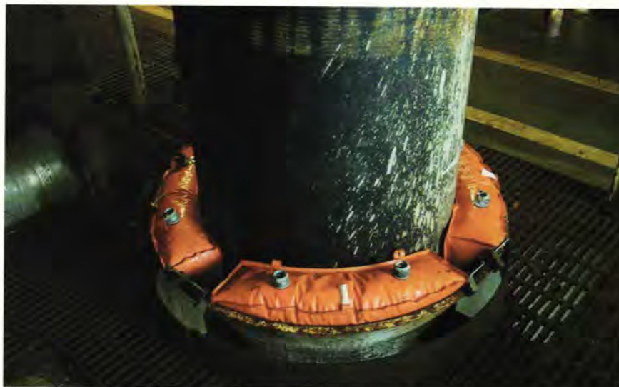
Smart-Shim chocks in position on BP Bruce
