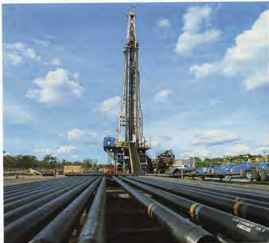
Production lines to be installed in one of the 300-plus wells drilled on the Sincor project in Venezuela
