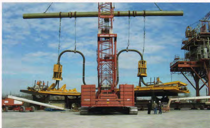
Top: A 16-inch to 20-inch diameter collet connector running tool being readied for systems integration testing (SIT). Bottom: A pipeline end terminal (PLET) and jumper undergo systems integration testing (SIT)
