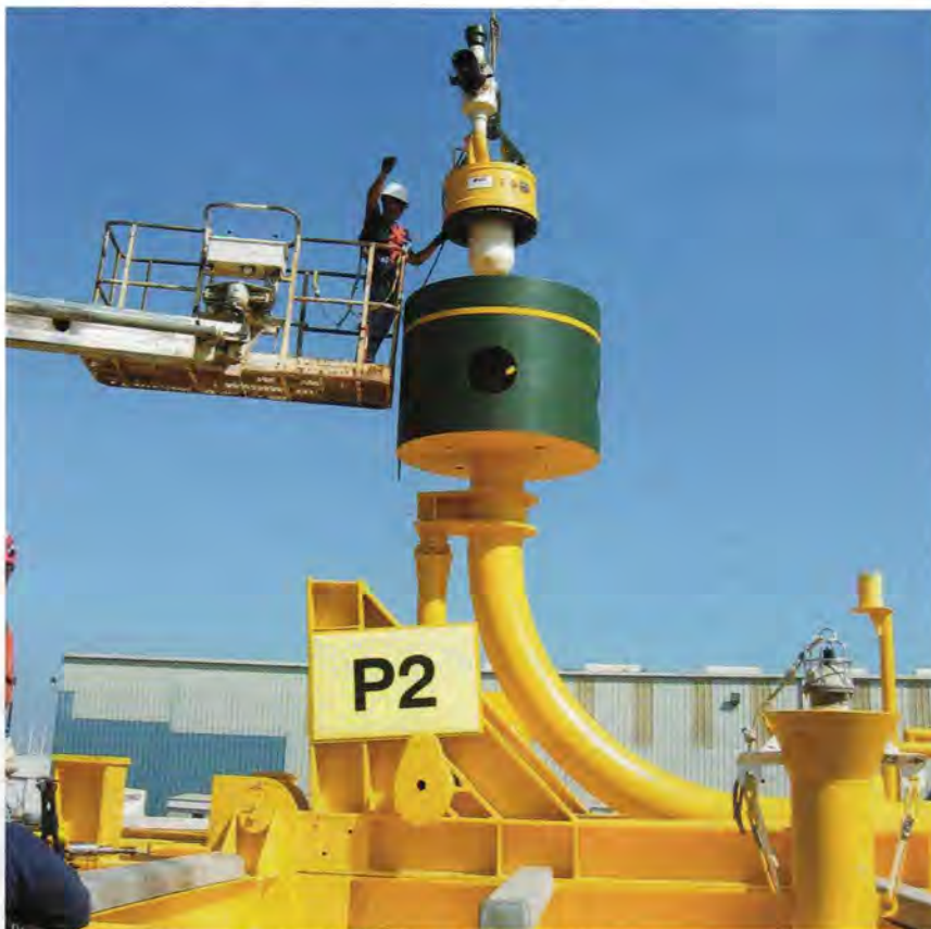
A pipeline end terminal (PLET) for the BP-operated Mardi Gras project undergoes system integration testing (SIT) at the Omega yard in New Iberia, La.
