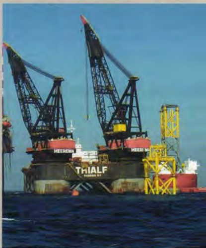
New facilities, including this flare-tower jacket, have been installed by Heerema crane-barge Thialf on Mærsk's Halfdan field this summer
