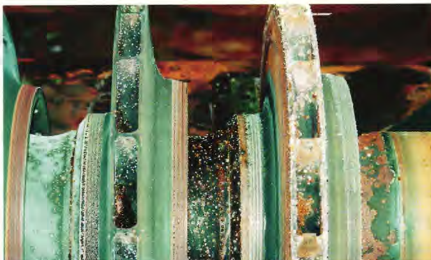
Fouled and corroded centrifugal compressor impellers
