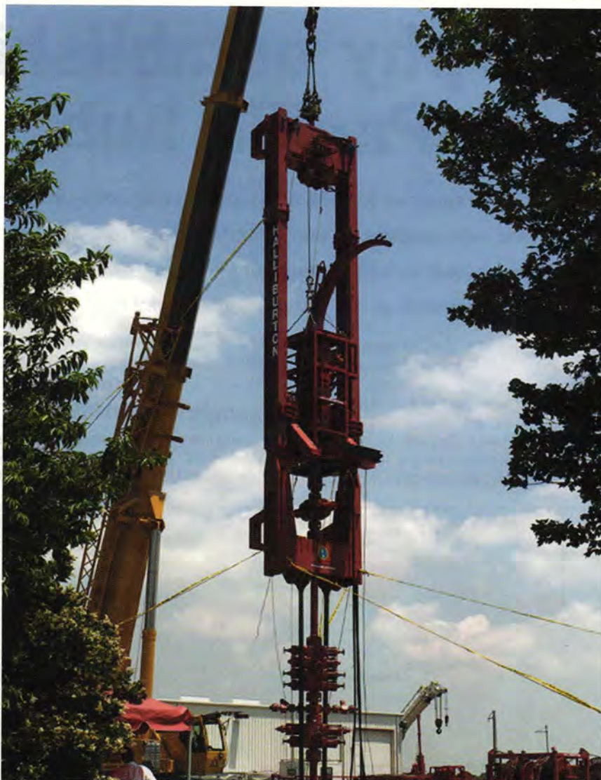
Injector frame for Thunder Horse coiled tubing system Photo: Halliburton
