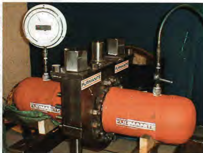
Pressure testing the leak-sealing clamp
