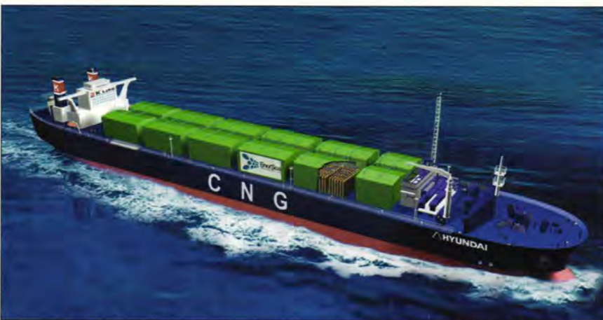
Figure 4: The EnerSea volume optimized transport and storage (VOTRANS) system delivers gas in long, large-diameter pipes in an insulated cold storage cargo package at low pressures. The design accommodates 700–800mn cf of natural gas, depending on the specific gas composition. EnerSea intends to use this vessel to support economic gas transportation services for applications with average supply rates ranging from 300–500mn cf/d of gas in markets up to 2,500 miles away.
