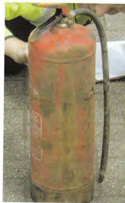
Fire extinguishers are important – unfortunately, the state of this one is not uncommon on UK vehicles
