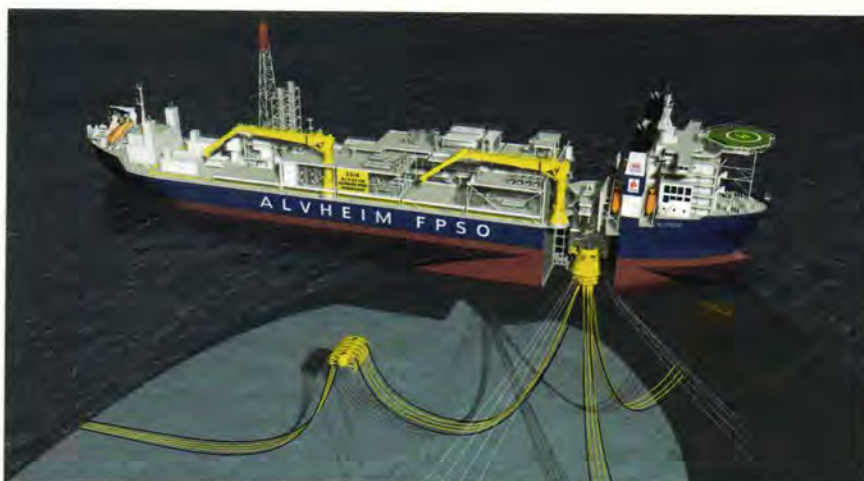
Figure 1: A submerged turret loading and mooring system supplied by APL will hook up the Alvheim FPSO to subsea wells Source: Marathon Oil
