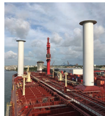
Trials of Flettner Rotor Sails have demonstrated they are one of the few ESTs expected to offer double-digit percentage improvements through auxiliary wind propulsion, and could play a key role in supporting the shipping industry to improve its environmental impact
