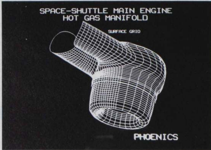
Fig 2: Representation of a space shuttle engine using the finite volume method
