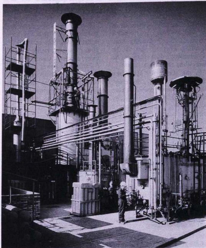
A furnace on the new Airoil Flaregas test rig being prepared for a performance trial.
