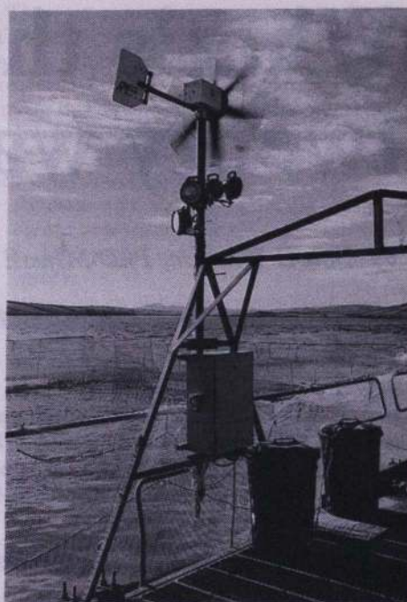
50 W wind turbine used to supply power for an automatic fish feeder.
