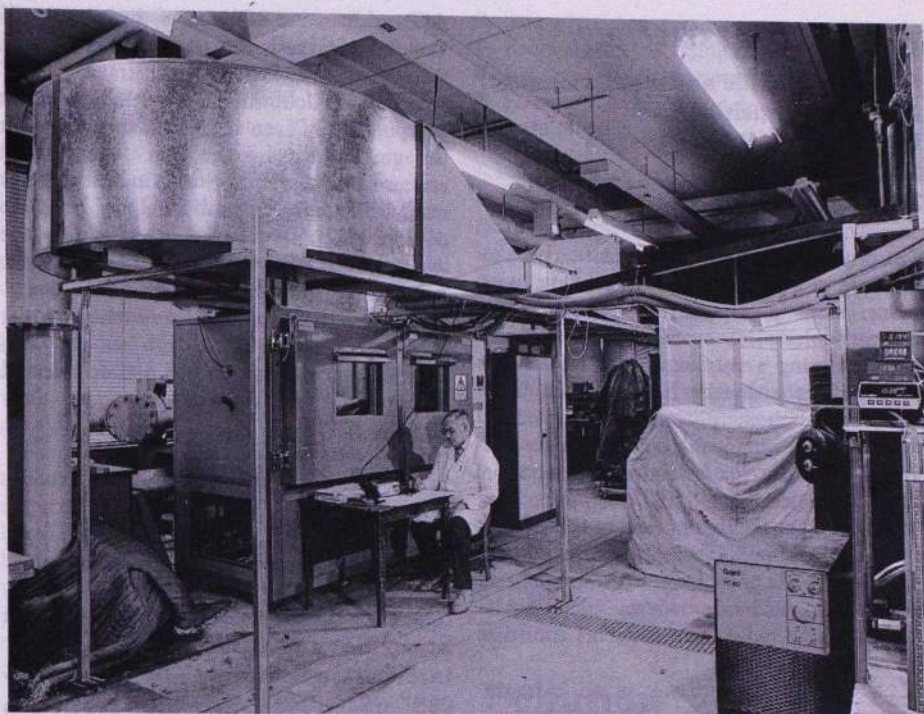
The fan-coil test facility, used for testing all fan-coil heating and cooling units under both design and worst case conditions of temperature and humidity.
