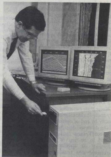
The Landmark third party system is an example of computer equipment becoming more compact. The process unit is little larger than a suitcase. An LP disc, being inserted, has a capacity equal to two million A4 sheets.
