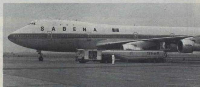
Figure 5(b) B747, Brussels low profile 65,000 Litre fueller
