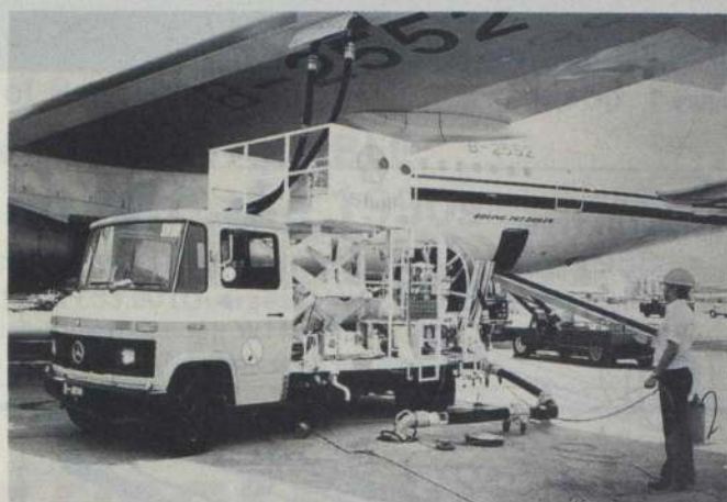
Figure 5a Shell 'Hart' 3800 litre/min hydrant dispenser fuelling B747 at Hong Kong
