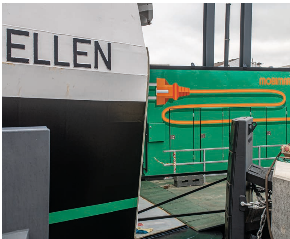
The Ellen electric ferry's battery capacity is 4.3 MWh Photo: Mobimar
