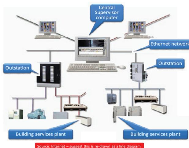
This allows the operator to program when things automatically turn on and off and what setting they operate at e.g. temperature, humidity. A BEMS is really a tool for controlling and monitoring the building and a good operator can use the BEMS to optimise settings to minimise energy consumption without compromising comfort and services.
